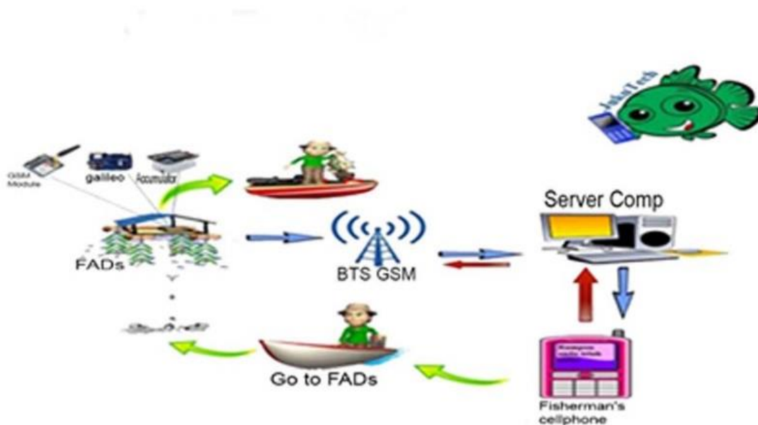
Figure 3. JukuTech Schematic ©2016 Merdeka.com
